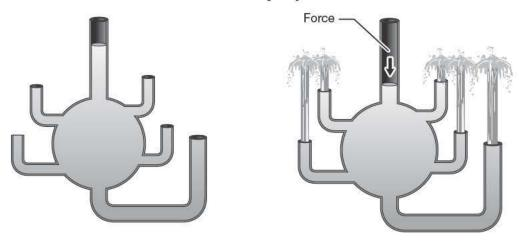
This is the principle that allows a hydraulic hoist to function.
