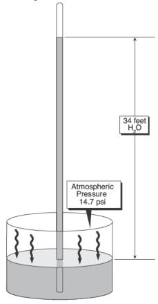
Therefore, the weight of a column of atmosphere is 14.7 psi which is equivalent to a column of water approximately 34 feet tall.
