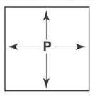
Pressure at any give point in a liquid at rest is the same in all directions. (If this were not true the liquid would be in motion.)
