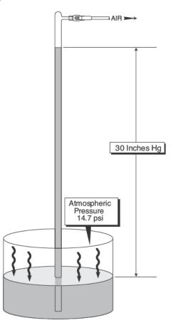
Based on the conversion of feet of head to pressure we can determine the pressure in psi of the atmosphere.
