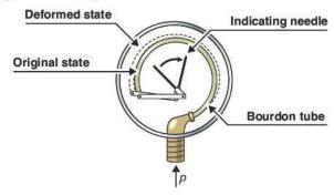
Dry gauges usually use the "C" shaped Bourdon tube. Liquid filled gauges usually use the helical or spiral Bourdon tube.
