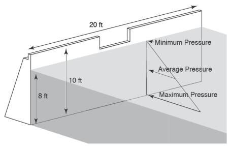
The average pressure is the pressure one-half the depth or 4 feet.
