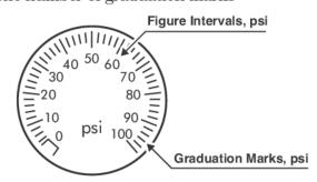
Figure intervals refer to the value between numbers on the dial face. Typical value differences are 1, 10, 25, and 100. The most common is 10. The dial face above has a figure interval of 10. That is, it is 10 psi between each number.
